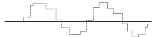
Greater deterioration of output signal and a time lag. Output Signal Deterioration
